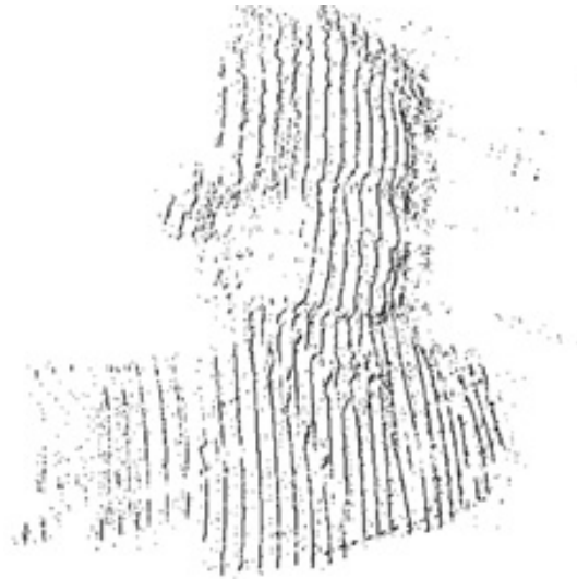
Figure 4.11: Triangulated point cloud with plane background masking and artifact elimination through meshing threshold=0.0.
