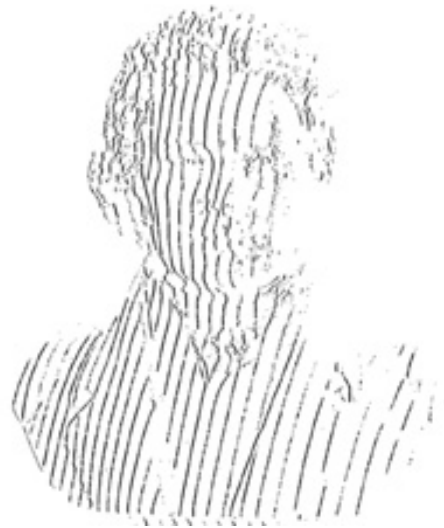
Figure 4.4: Edge detection with restricting 5 consecutive edge pixels and threshold=0.002.
