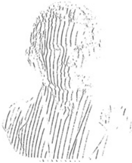
Figure 4.5: Edge detection with restricting 7 consecutive edge pixels and threshold=0.002.
