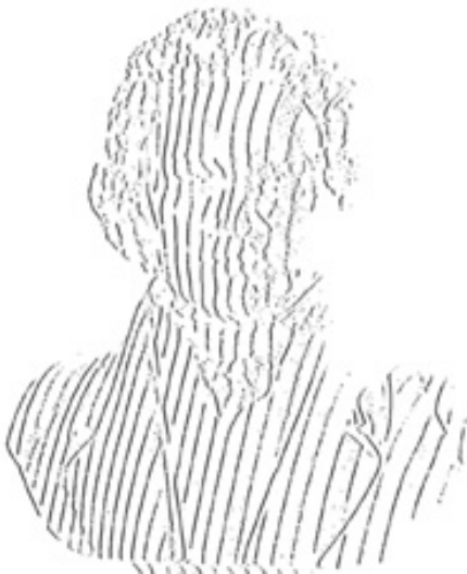
Figure 4.7: Edge detection with restricting 10 consecutive edge pixels and threshold=0.001.
