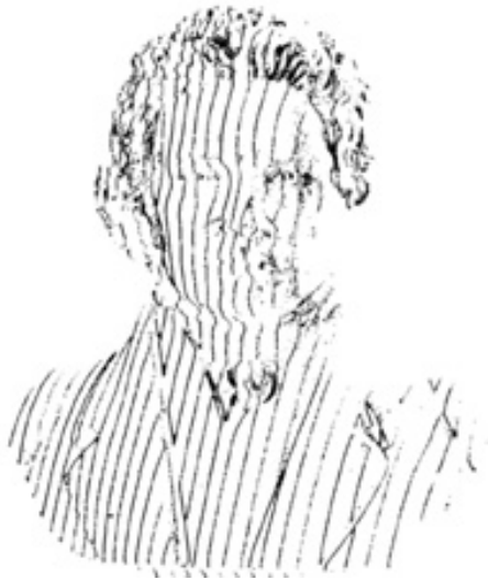
Figure 4.3: Edge detection without consecutive edge pixel restriction and threshold=0.002.
