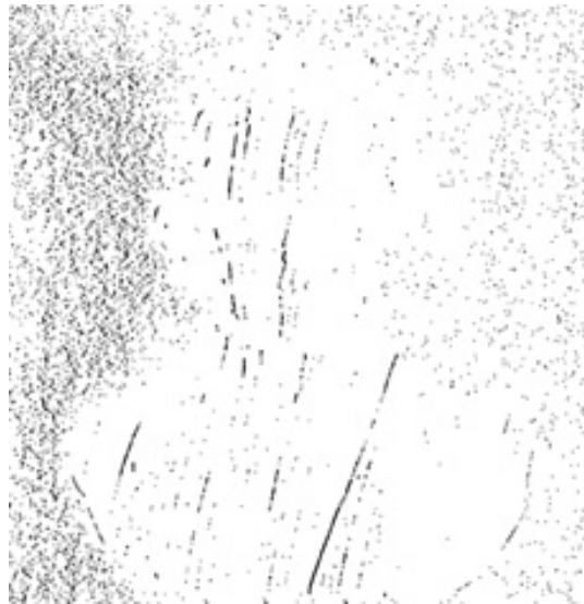
Figure 4.8: Edge detection with restricting 10 consecutive edge pixels and threshold=0.000.
